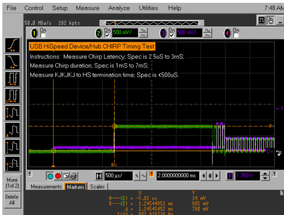
Using the automatic measurement shown in Figure 14, measure the device's CHIRP-K duration.
