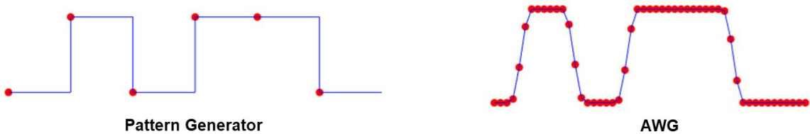
Figure 4 Effects of applying pulse shaping filter
