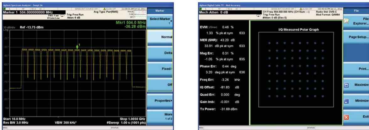
Figure 95: 84 64QAM DVB-C signals being generated simultaneously by an AWG (A Keysight M8190A). Notice the excellent available dynamic range and the lack of spurs (left) and the modulation quality obtained (right) with EVM lower than 0.5%.
