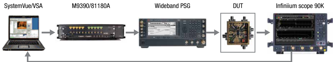
Figure 5.2. SystemVue, in combination with best-in-class AWG and oscilloscope test families, provides a closed-loop, stimulus/response modeling, and verification platform up to 32 GHz wide. It enables a versatile and cost-effective UWB system-level approach in R&D.
