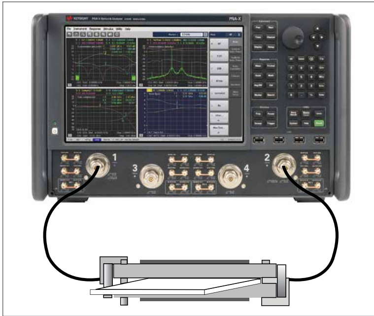
Figure 15.7. Resonant cavity method with network analyzer
