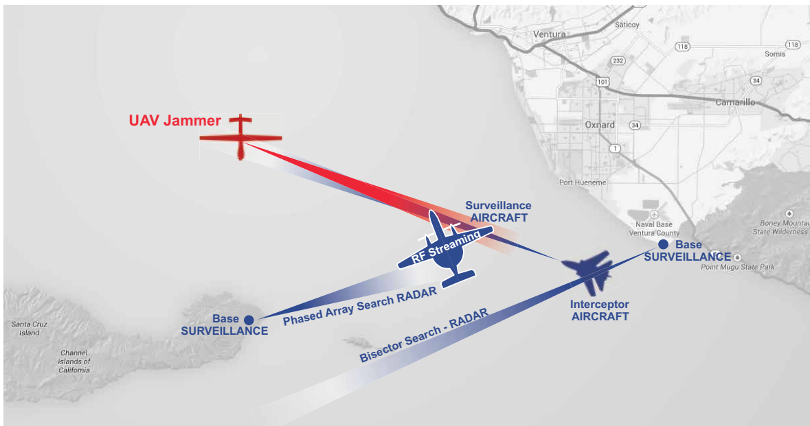
Figure 22.6. An RF streaming solution is placed on-board an E2-C to record the interaction between interceptor radar and jamming response from the UAV.
