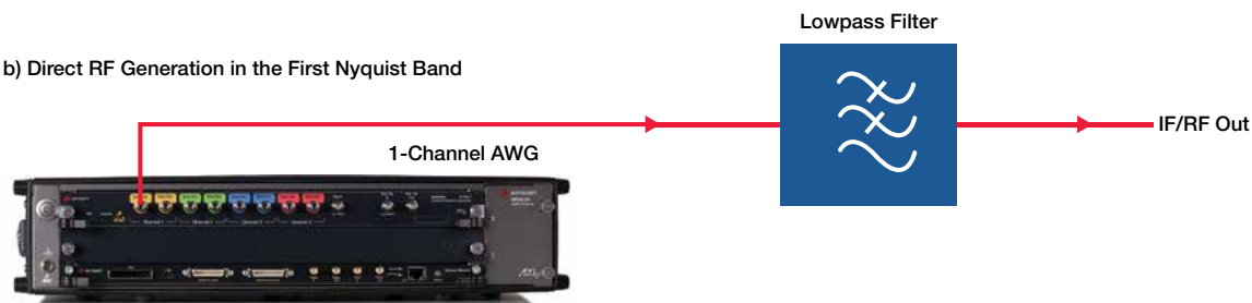
Figure 16.10. AWGs can generate radar (and any RF) signals following to different basic schemes
