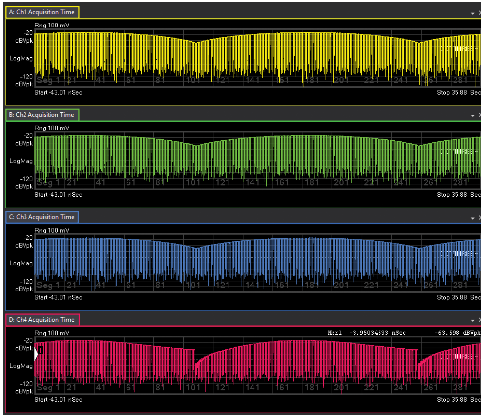
Figure 17.21. Segmented capture across four channels
