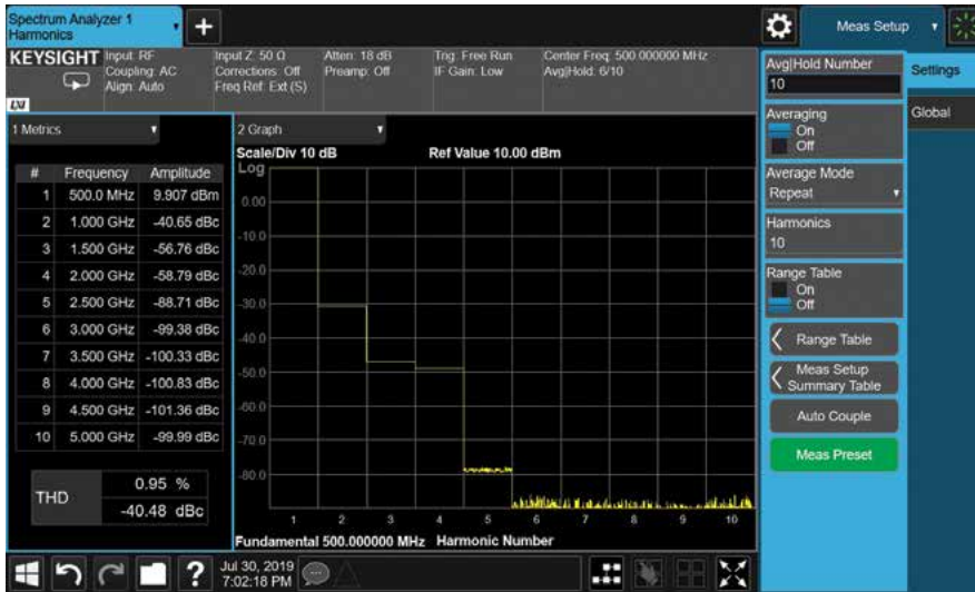
Figure 9.2. Harmonics measurement with Keysight signal analyzer
