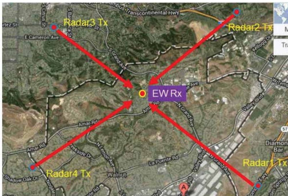
Figure 20.8. Shown here is an example of an ew receiver test environment with several geographically dispersed emitters contributing to signal conditions at a centrally-located receiver.
