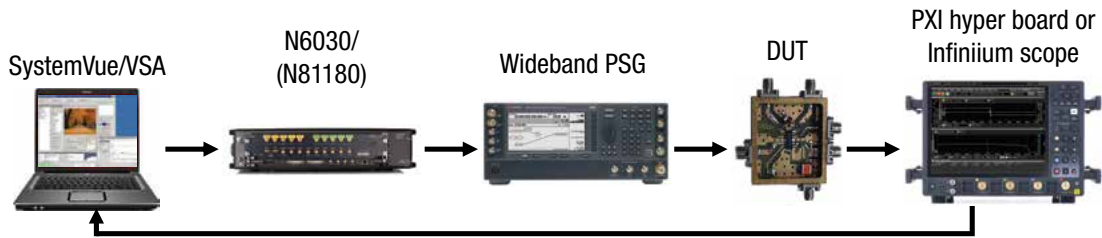
Figure 7.10. Test setup for wideband signal generation.
