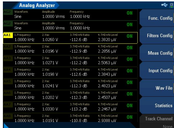
Figure 1. The U8903B's GUI, showing 8 analyzer channel measurements.
