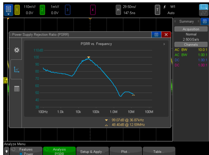
Figure 37. Power supply rejection ratio (PSRR) measurement using the scope's built-in waveform generator as an automatic swept source.
