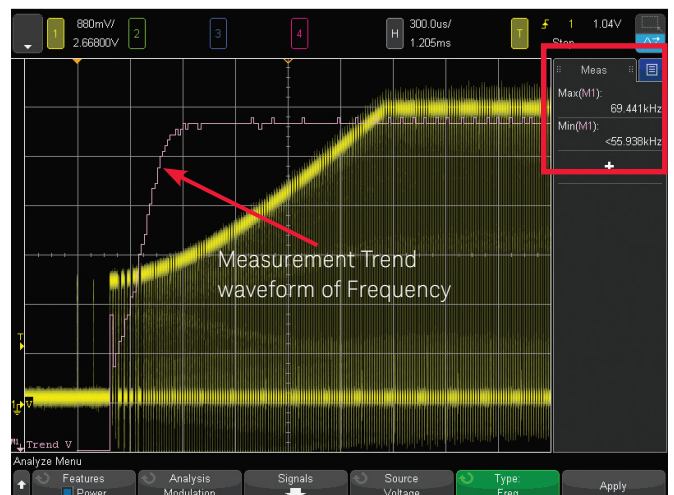
Figure 26. Modulation measurement of frequency on the switching transistor's Gate input during power-up.
