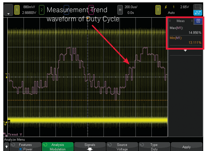
Figure 25. Modulation measurement of duty cycle on the switching transistor's Gate input.
