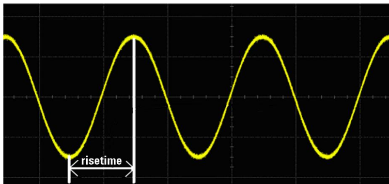
Figure 24. An example of risetime (0 to 100% of peak-to-peak voltage is shown instead of the usual 10 to 90%).
