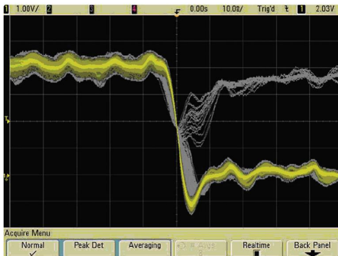
Figure 19. An infrequent glitch caught on a Keysight InfiniiVision 6000 Series oscilloscope.
