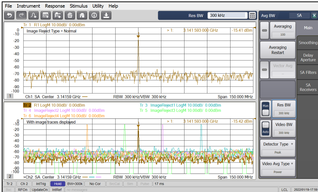
Figure 37. Normal image rejection (top) and special diagnostic mode showing the image signals (bottom).
