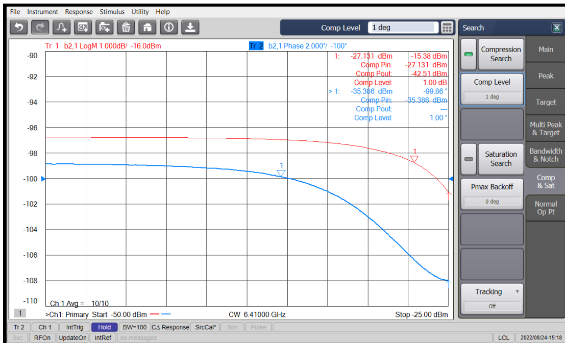
Figure 18. Example phase-transfer measurement resulting from a power sweep of an out-of-band signal.
