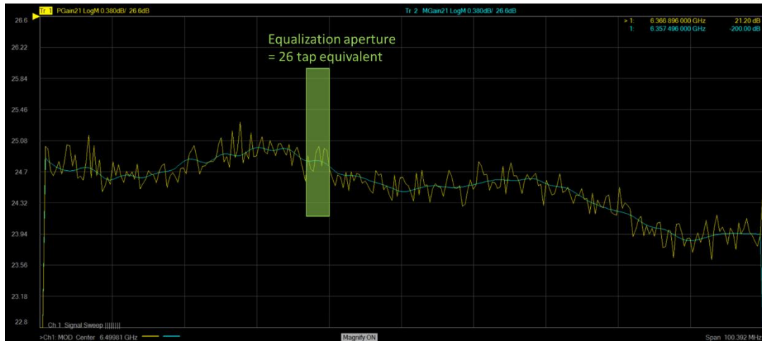
Figure 30. An appropriately set equalization aperture shows the MGain trace following ripples in the DUT output
