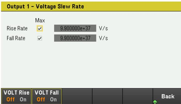
1. Configure the **Rise Rate** or **Fall Rate** accordingly. Use the navigation keys to select the field; use the numeric entry keys to enter the value. The value is set when you press **[Enter]**. You can also enable the **Max** checkbox to set the slew rate to the maximum value.
