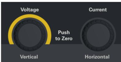
These knobs are active in Meter View, Scope View, Data Logger View, as well as in Settings page.
